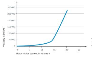
Viscosity measurement by Brookfield DV2-T at 23 °C and 10 RPM in epoxy systems Araldit® casting resin (Carl Roth) spindle 5/7
