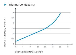
Thermal conductivity measurement via THB 100 in epoxy systems Araldit® casting resin (Carl Roth)
