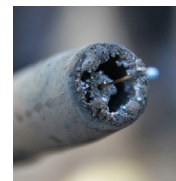
Welding nozzle without HeBoCoat® SL-E 125 coating.
