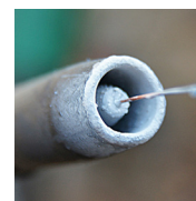
Welding nozzle with HeBoCoat® SL-E 125 coating.
